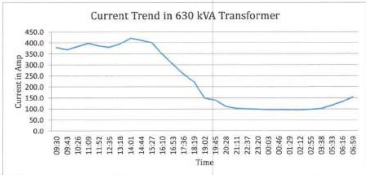
Figure 2: Current Trend of LT side of transformer
